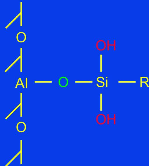
A basic mechanistic model for silane deposition on active substrates was described by Arkles (Ref 1). Figure 7 shows its main elements. The alkoxysilane is first hydrolyzed to generate active silanol intermediates. These intermediates partially oligomerize in solution. The illustrated model shows a partially oligomerized trimer approaching the substrate surface. Hydrogen bonding initially occurs, followed by elimination of water on thermal cure, generating a stable Si-O-Si covalent bond.
