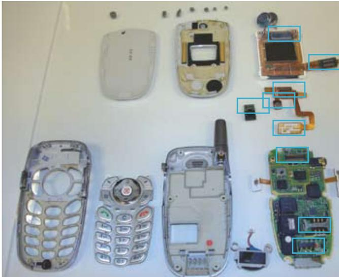
Disassembled Phone – Connectors Highlighted
