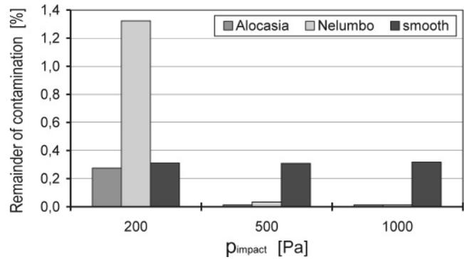
**Figure 4.** Remainder of contamination on replicates of two plant surfaces and one smooth surface made of a hydrophobic polymer after sprinkling with water drops. The kinetic energy and, therefore, the impact pressure of the drops were varied.**Table 7. Contact Angle (Mean Value  $\pm$  Standard Deviation)  $\theta$  of Perfectly Smooth Silicon Chips Hydrophobized with Different Agents and of a Smooth Surface of the Polymer Used for the Replicates**
