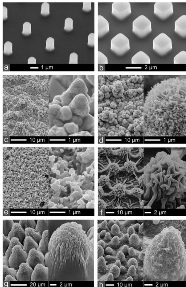
**Figure 1.** (a–h) SEM photographs of microstructured water-repellent surfaces: (a, b) silicon chips with regular patterns of spikes, (c) copper foil *Cu-1*, (d) copper foil *Cu-2*, (e) aluminum foil *Al-1*, (f) replicate of *Alocasia*, (g) replicate of *Rosa*, and (h) replicate of *Nelumbo*.
