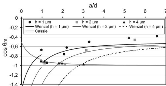
**Figure 2.** Water contact angles  $\theta_m$  of hydrophobized silicon chips with regular patterns of spikes (whose width  $d$ , clearance  $a$ , and height  $h$  were varied) as a function of  $a/d$ , compared with the plots of  $\theta_m$  for Wenzel and Cassie drops. For  $a/d < 1$  the calculations were made for spikes with a 2- $\mu$ m-wide square base, and for  $a/d > 1$  the spikes represented 0.9- $\mu$ m-wide cylinders.
