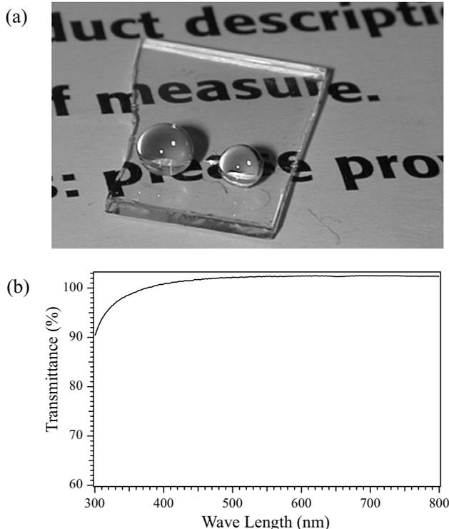
**Figure 8.** (a) Photograph of water droplets placed on the film prepared on the glass substrate. The film was deposited at the value of  $R$  of 0.25. (b) Visible light transmittance of the film prepared at  $R = 0.25$ .
