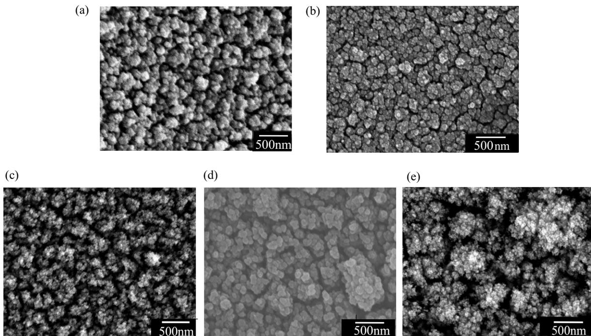
**Figure 3.** FE-SEM images of nanotextured surfaces deposited by MPECVD with different values of  $R$ . (a)  $R = 0$ , (b)  $R = 0.25$ , (c)  $R = 0.5$ , (d)  $R = 0.75$  and (e)  $R = 1.0$ .
