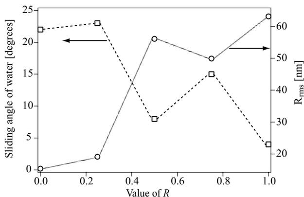
**Figure 4.** The relationships between sliding angles for water drops, the surface roughness ( $R_{rms}$ ) and the value of  $R$ .
