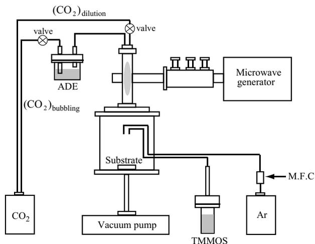
**Figure 1.** A schematic illustration of the MPECVD apparatus.
