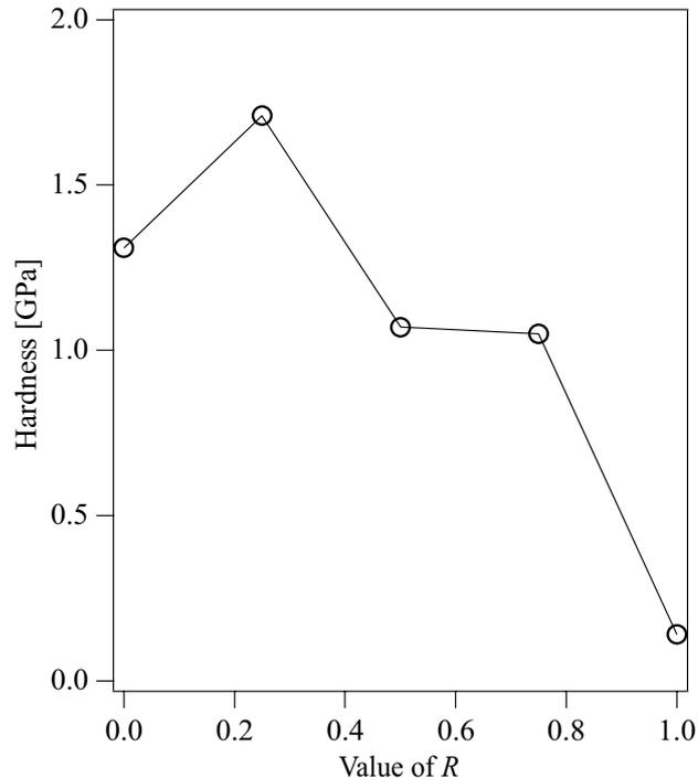
**Figure 7.** Hardness of the deposited films at various values of  $R$ .
