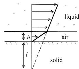
Fig. 6. Slip length and velocity distribution in a liquid flow over a gas film near a solid wall. Since gas viscosity is much smaller than that of the liquid, the observed slip length  $l$  has a finite value given by Eq. (18).
