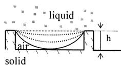
Fig. 2. Destabilization of the composite interface due to increasing amplitude of a liquid–air interface capillary wave. If wave amplitude is high enough so that it touches the valley between asperities, the liquid can fill the valley.
