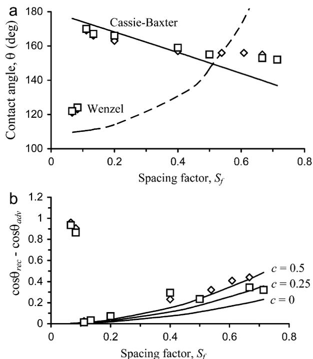
Fig. 7. (a) Static CA  $\theta$  as a function of the spacing factor  $S_f$  for the first (squares) and the second (diamonds) series of the experiments compared with the Wenzel and Cassie–Baxter models. (b) The values of  $\cos \theta_{rec} - \cos \theta_{adv}$  as a function of  $S_f$  for the first (squares) and the second (diamonds) series of the experiments compared with the theoretically predicted values (solid line).
