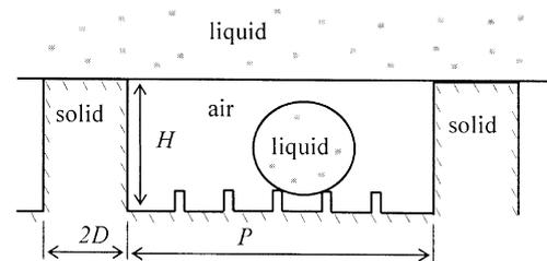
Fig. 5. Schematic of a rough surface with pillars. Smaller scale roughness is required to support small size droplets.
