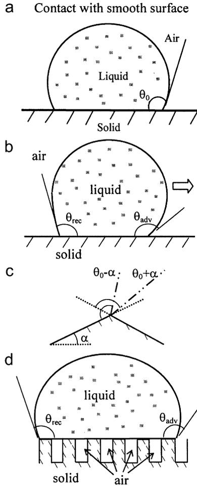
Fig. 1. Liquid droplet in contact with (a) smooth profile (the value of CA is  $\theta_0$ ), (b) rough profile (the values of advancing and receding CA are  $\theta_{adv}$  and  $\theta_{rec}$ ), (c) sharp edge (the values of CA may vary between  $\theta_0 - \alpha$  and  $\theta_0 + \alpha$ ), and (d) rough profile with composite interface.
